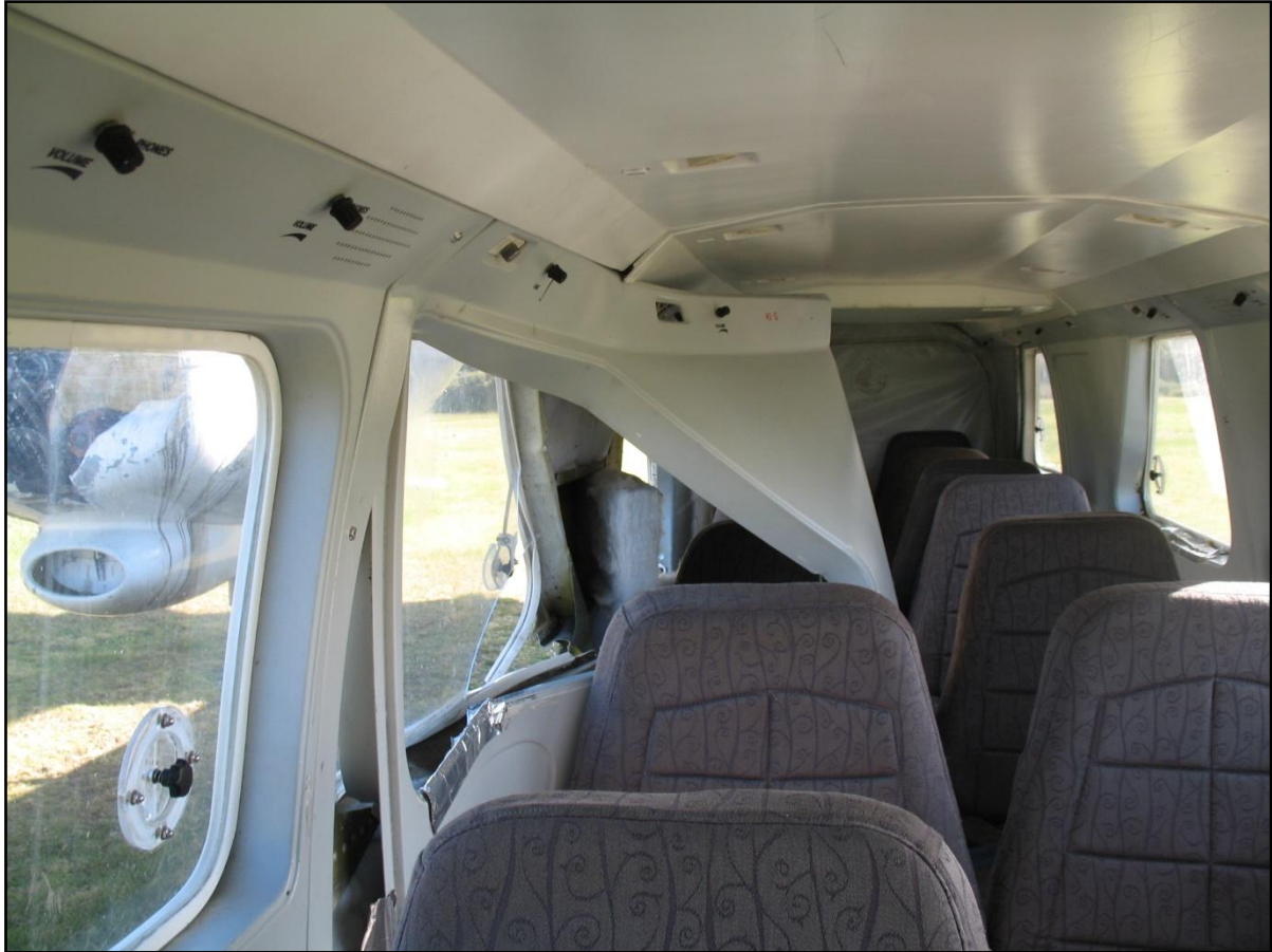
Figure 3 ZK-LOU interior showing cabin lining damage
