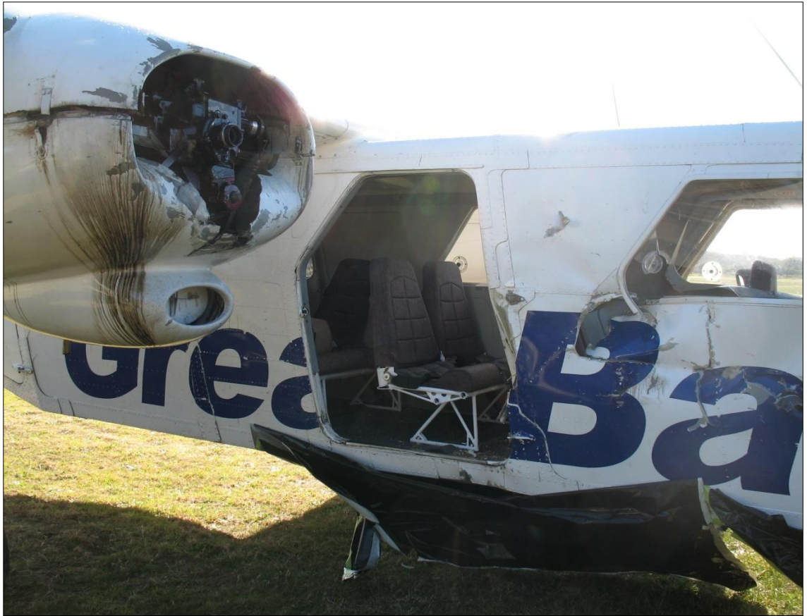
Figure 2 ZK-LOU right side showing damage and missing propeller
